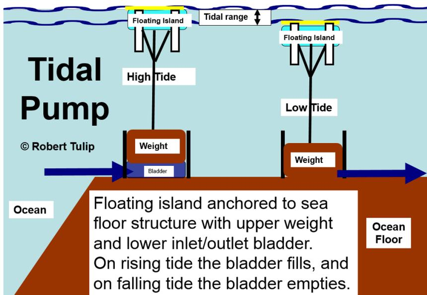
concept is only proved at the level of informal expert peer review. My concept for this tidal pumping method has had no formal research validation, although my informal discussions with hydrologists indicate it is feasible. The Tidal Pump uses a floating island to cause a weight on the ocean floor to rise and fall with the tide. The weight is anchored above an inlet/outlet bag on the ocean floor. The weight is
