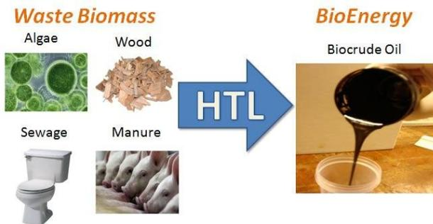
Hydrothermal Liquefaction is described as follows by researchers at the University of Illinois: “High moisture biomass is subjected to elevated temperatures (250-350° deg C) and pressures (10-20 MPa) in order to break down and reform the chemical building blocks into a bio-crude oil. At these temperatures and pressures, water becomes a highly reactive medium promoting the breakdown and cleavage of chemical bonds, allowing for the reformation of biological
